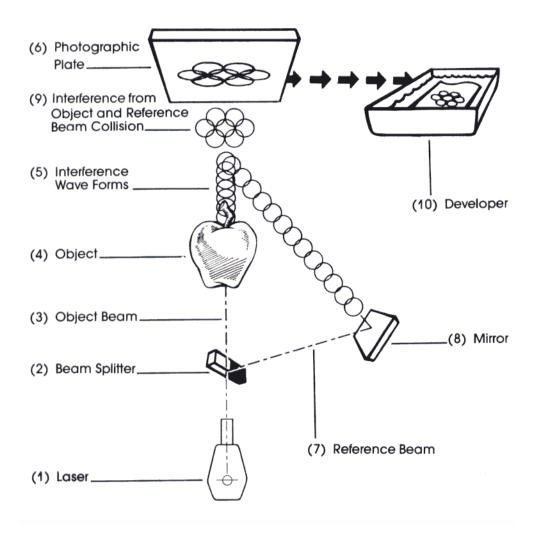
Looking at the developed film plate, the naked eye barely perceives the unintelligible swirling gray and white interference patterns created by the collision of the object and reference beams of light. (Refer to the illustration on the next page.)
